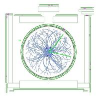
Muon candidates reconstructed in the Central Outer Tracker(COT) and Central Muon detectors(CMU,CMUP).
