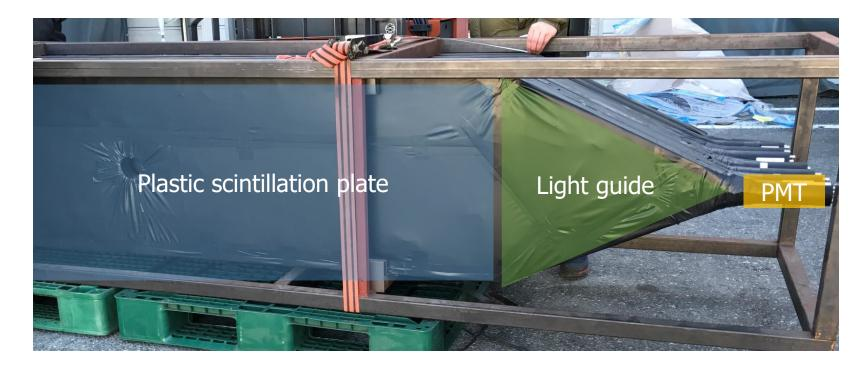
Plastic scintillation plates x 9 : 250\*60\*5 [cm<sup>3</sup>] 2" PMT x 18 : 2 PMT on both side of plate
