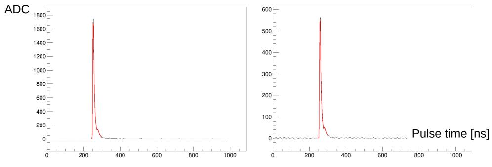
Pulse at center (-0.85 m  $\sim$  -0.80 m), Left PMT
