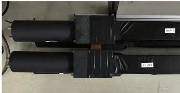
Figure 2: Pictures of the counters – attached PMTs and bars with bakelite guides ↵
