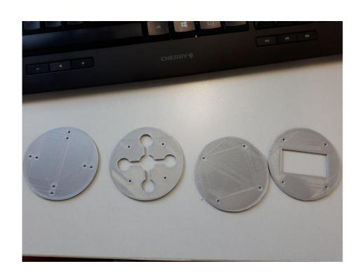
Support frame of new detector is made by 3D print
