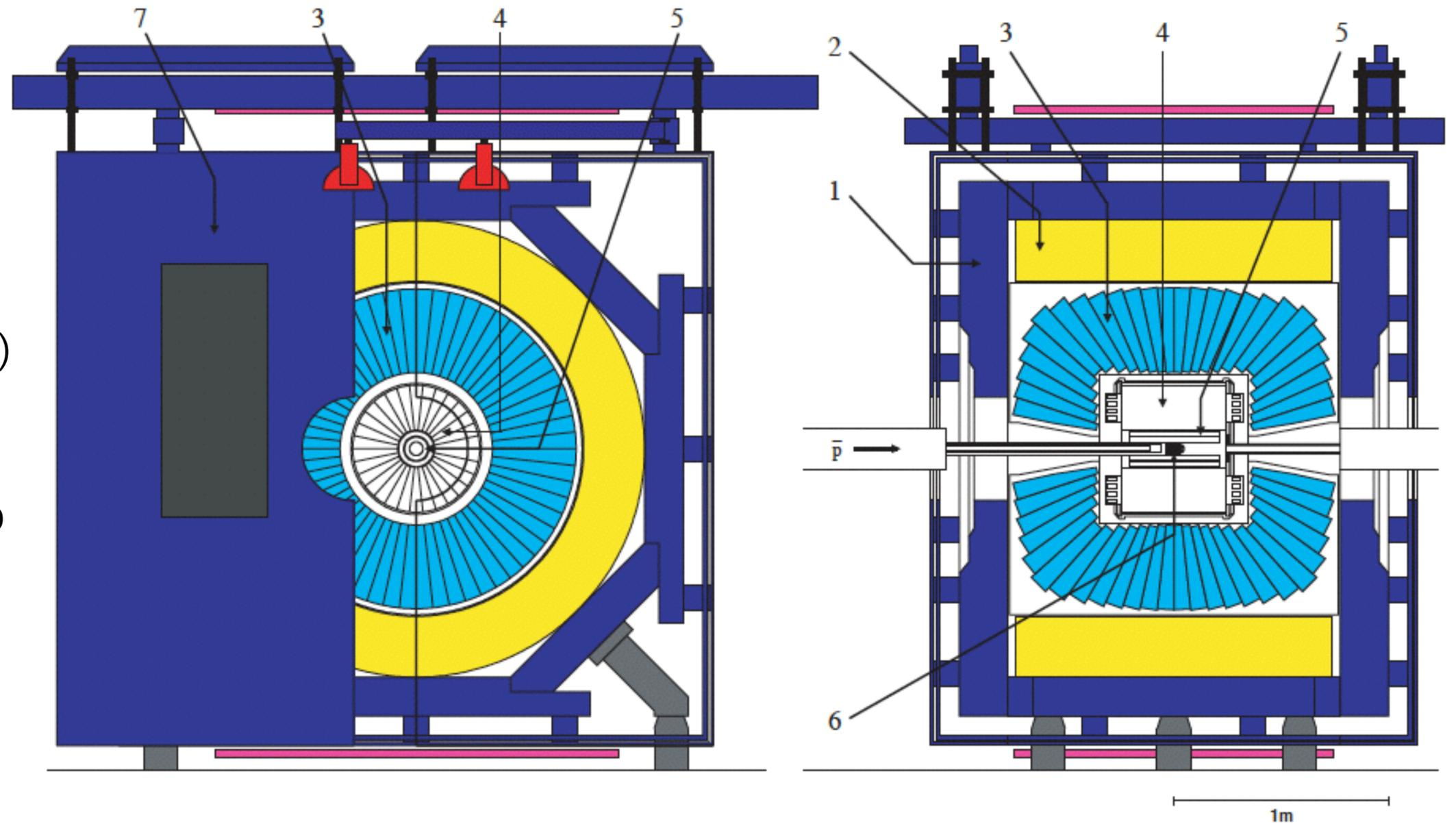
Fig. 4. Overall layout of the crystal barrel detector showing (1) magnet yoke, (2) magnet coils, (3) CsI barrel, (4) jet drift chamber, (5) proportional chamber, (6) liquid hydrogen target, (7) one half of endplate. Left—longitudinal cross section; Right—transverse view.
