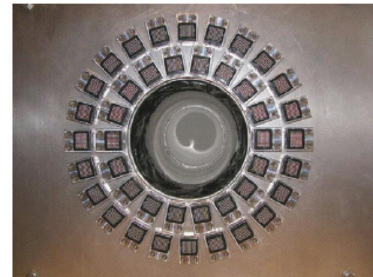
**Fig. 6.** The last plate with the PMTs inserted in their masks.
