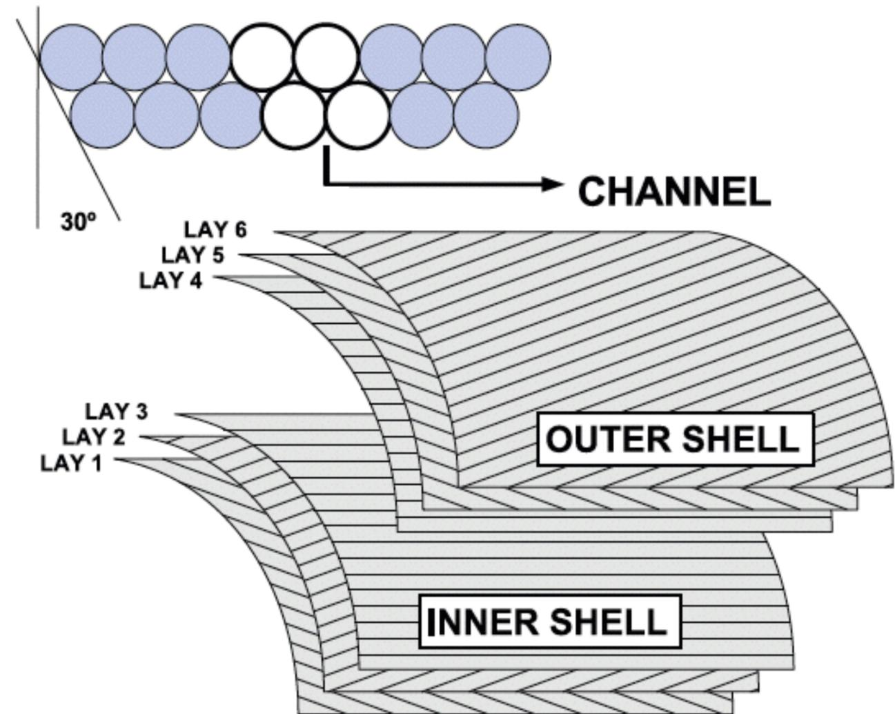
**Fig. 2.** Layout of the vertex detector; top drawing: zoom on a layer.
