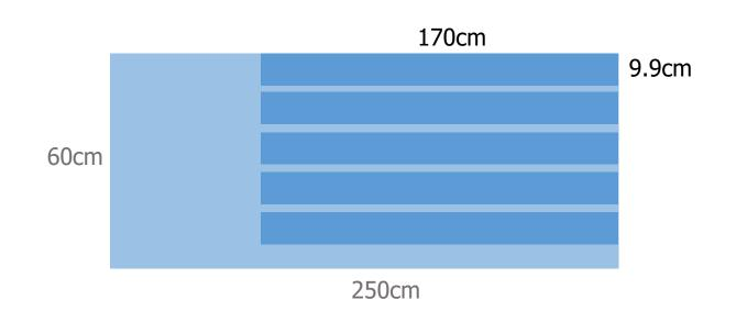
8 plates  $\rightarrow$  40 bars 1 plate with a hole  $\rightarrow$  4 bars
