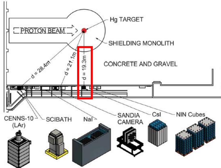
**Fig. 2. COHERENT detectors populating the “neutrino alley” at the SNS.** Locations in this basement corridor profit from more than 19 m of continuous shielding against beam-related neutrons and a modest 8 m.w.e. overburden able to reduce cosmic ray-induced backgrounds, while sustaining an instantaneous neutrino flux as high as  $1.7 \times 10^{11} \nu_{\mu} \text{ cm}^{-2} \text{ s}^{-1}$ .
