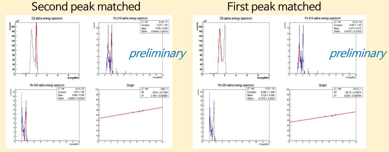
Get quenching factor using Po-210, Rn-220, Po-216 (first linear polynomial)
