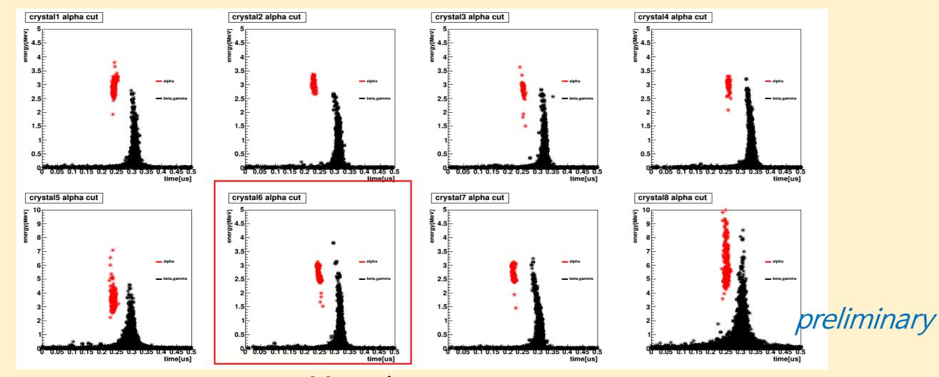
energy[MeV] Analysis high energy events to select alpha-alpha coincidence events Because Q value of Po-210 is 5.4 MeV
