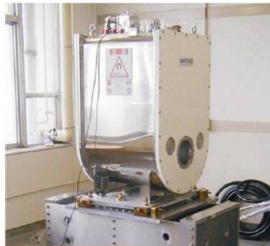
Figure 3.40: A photograph of the superconducting magnet of the cusp trap.
