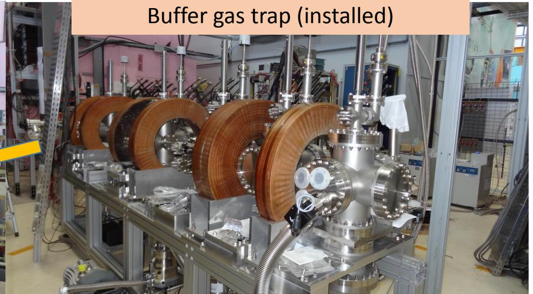
Buffer gas trap (installed)
